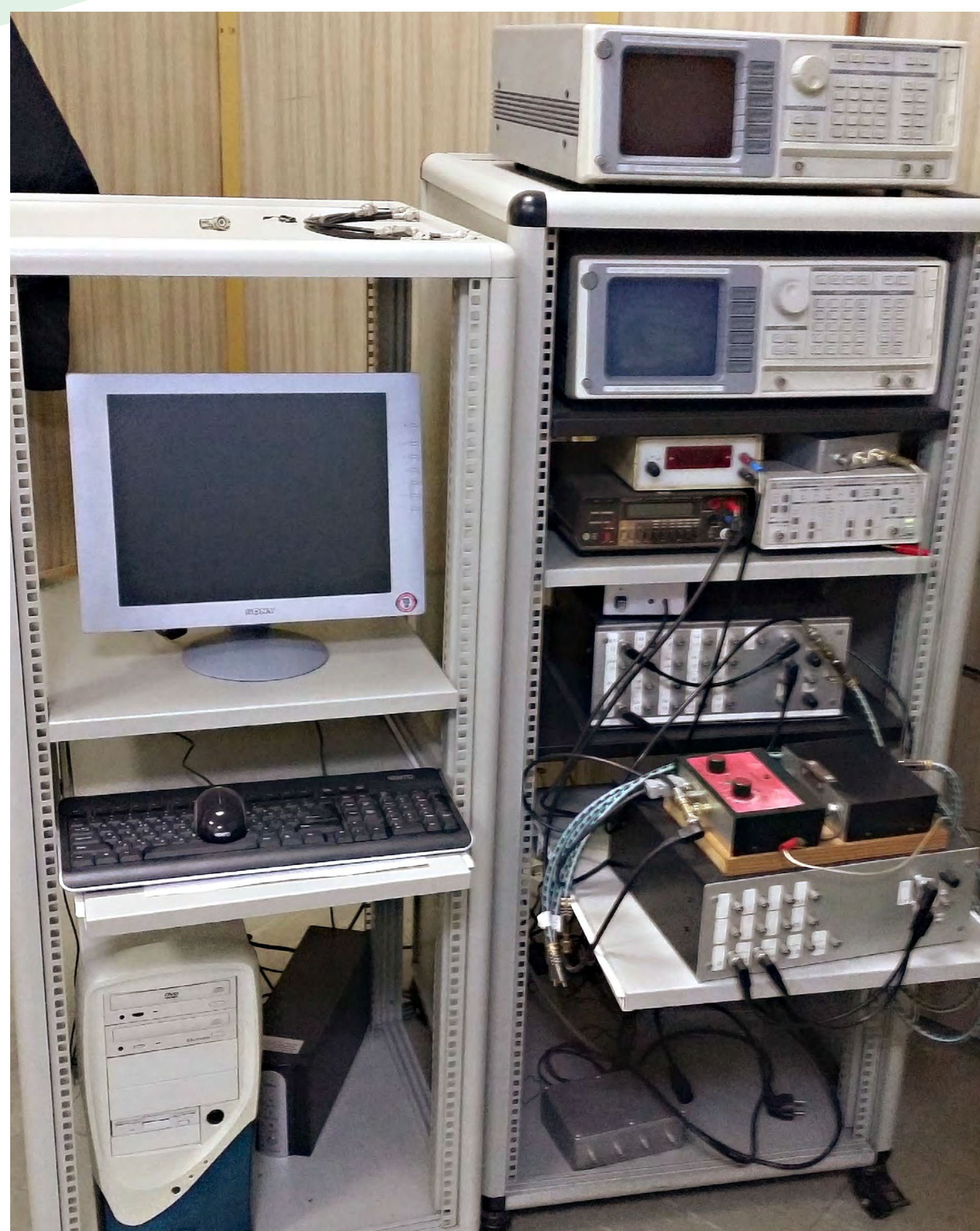
Computer controlled Low-Frequency Noise measurement system (1 Hz-100 kHz). It comprises two SR760 FFT spectrum analyzers and two SR570 low-noise current pre-amplifiers. All the critical stages are powered by NiMh batteries or are opto-isolated to reduce external noises and interference. The LFN technique allows for the characterization of carrier traps in semiconductor devices and materials.
