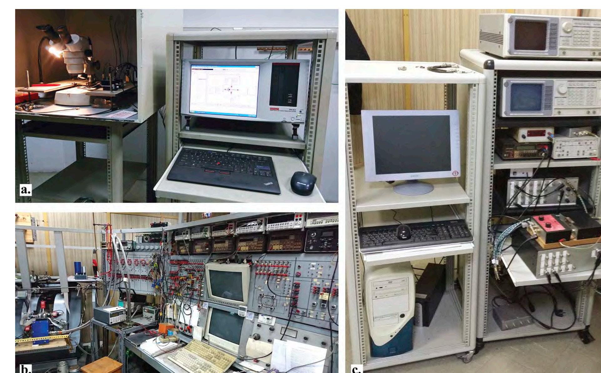
(a) Semiconductor characterization system Keithley 4200-SCS for electrical characterization of micro and nano-devices. (b) Van der Pauw and Hall measurements set-up (10-330 K & ≤ 1.4 T). (c) Characterization of carrier traps in semiconductor devices and materials, with a computer controlled Low-Frequency Noise (LFN) measurement system (1 Hz-100 kHz), with two SR760 FFT spectrum analyzers and two SR570 low-noise current pre-amplifiers
