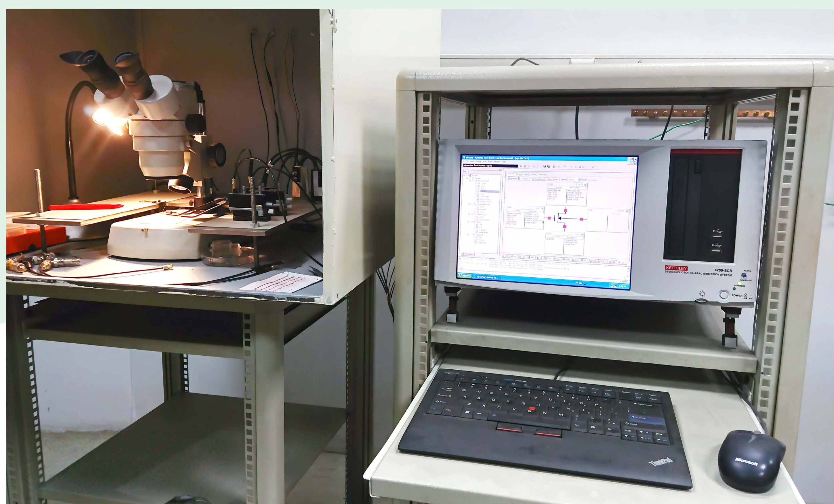
Keithley 4200-SCS (semiconductor characterization system) including I-V measurements and C-V spectroscopy, for electrical characterization of micro and nano-devices (2-4 terminals).
