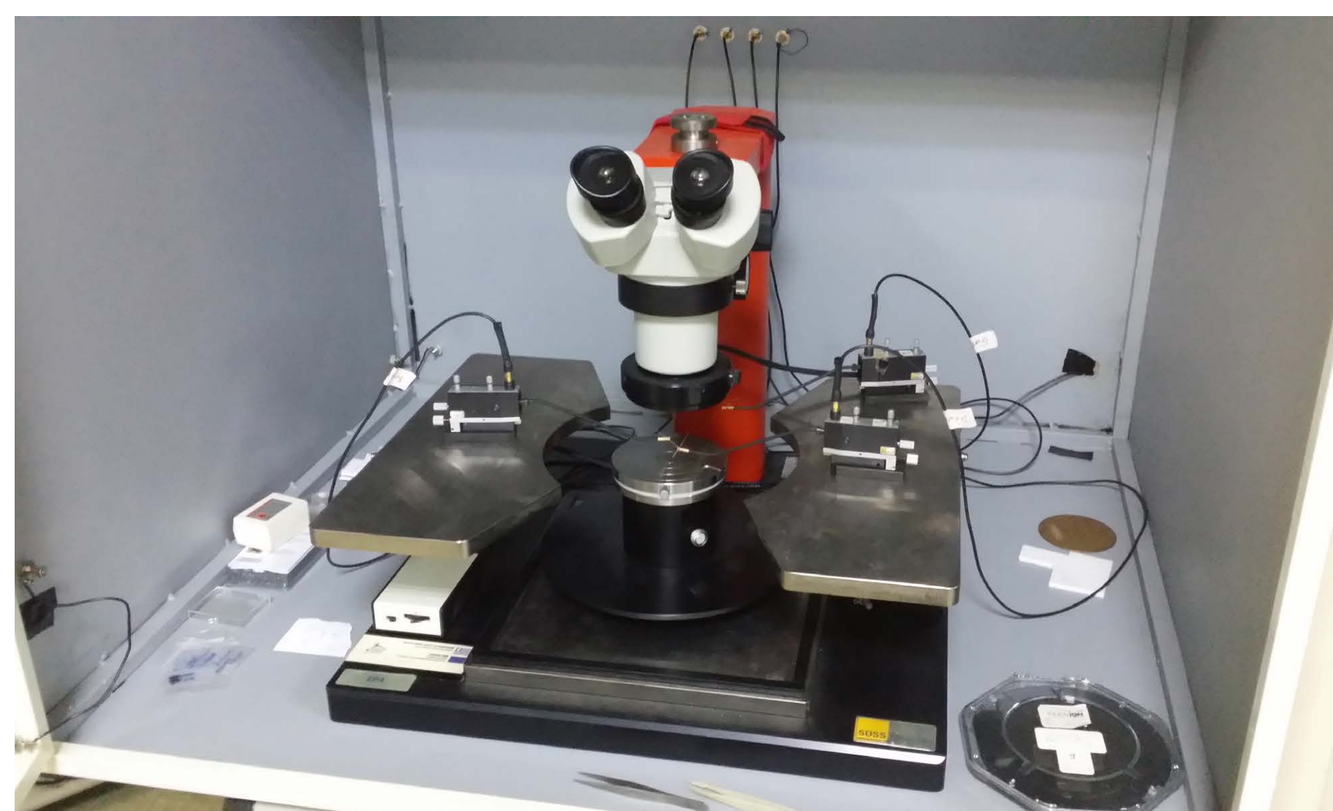
Probe station SussMicrotec EP4 for electrical contacts in "on-chip" semiconductor devices and integrated circuits.
