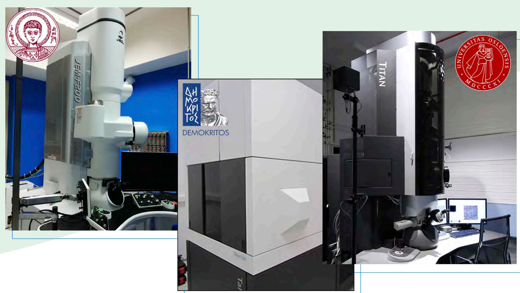
Advanced Scanning Transmission Electron microscopes located in the associated labs. From left to right:
