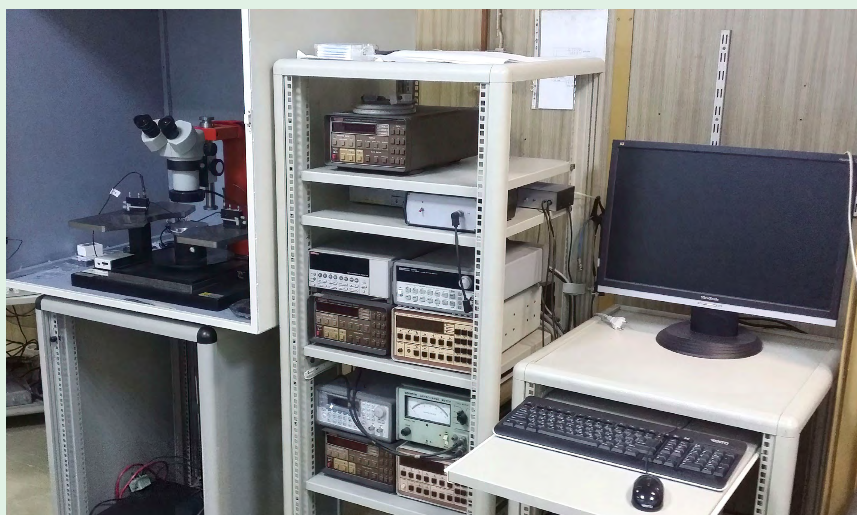
Computer-controlled system for I-V and C-V measurements, to fully characterize modern transistors or diodes. The system comprises voltage, current sources and arbitrary pulse generator, thus is capable for studying also Hot-Carrier effects (static & dynamic electrical stress).
